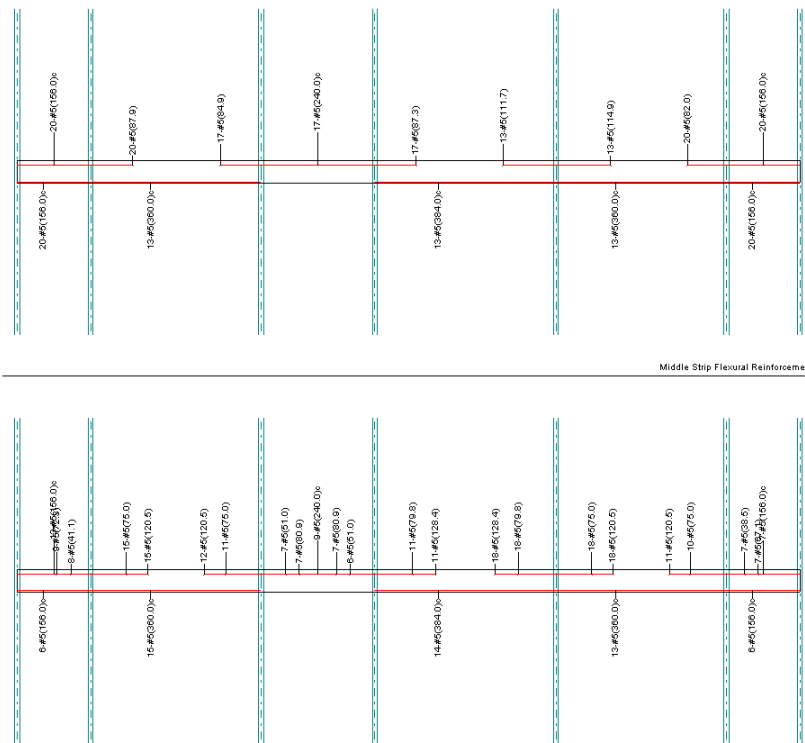
Figure 27 –Reinforcement for Typical AHU Width
