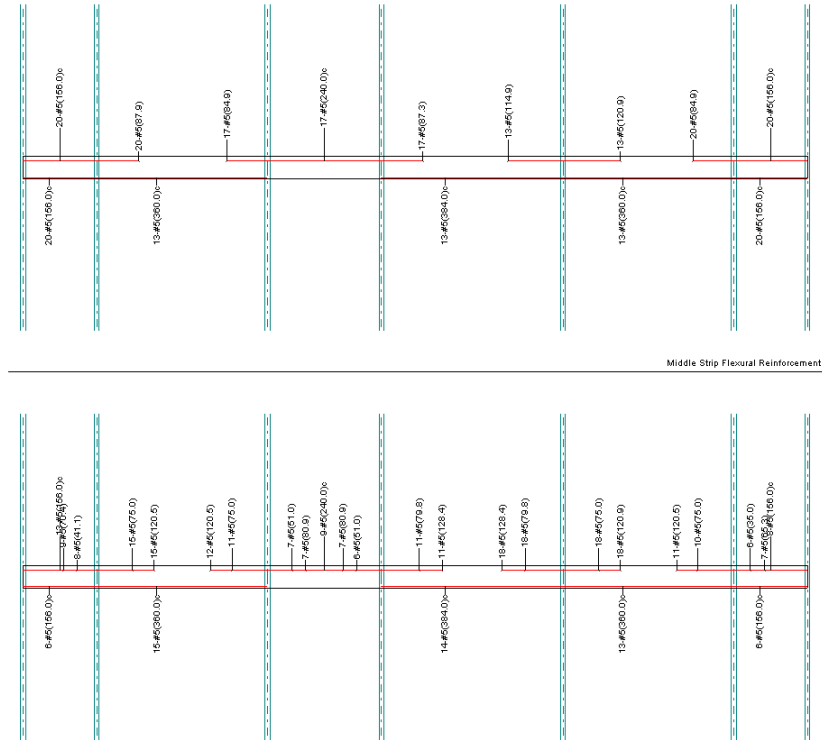
Figure 30 –Reinforcement for Typical Cooling Tower Width
