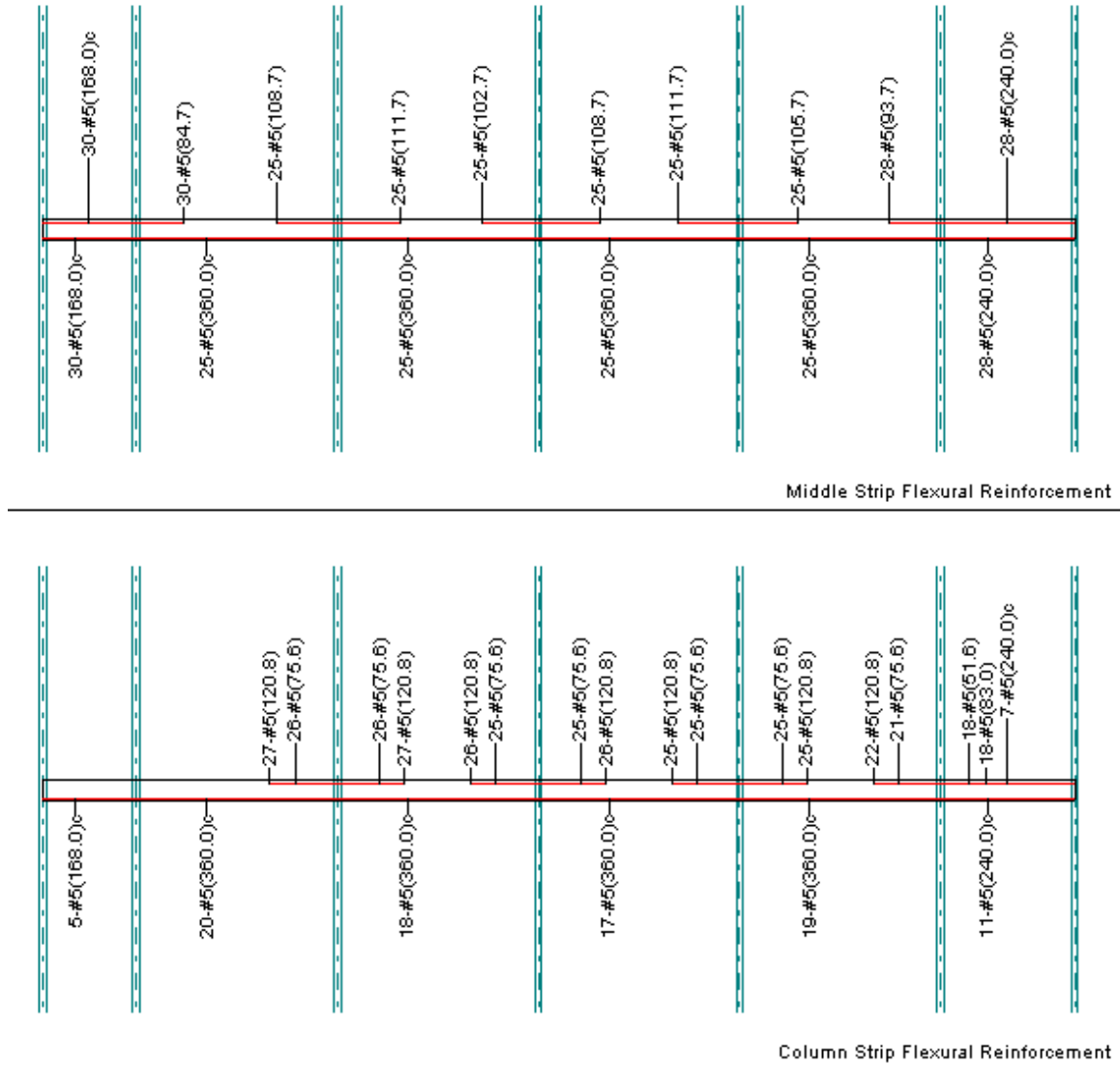
Figure 37 –Reinforcement for Typical Cooling Tower Length
