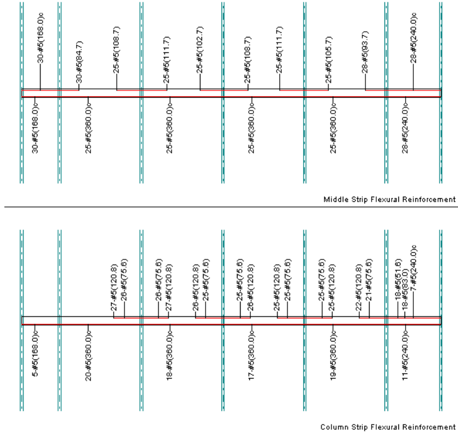
Figure 34 –Reinforcement for Typical AHU Length
